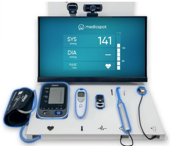
Image shows diagnostic toolkit available for in-pharmacy consultations. These include, blood pressure cuff, medical camera, stethoscope and blood oximeter
